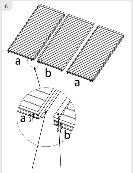
When assembling the shutter walls, Note the side tube direction:
