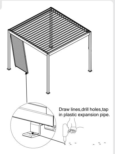
If the floor is a wood floor, you don't need to knock in the plastic expansion pipe, directly use J to knock
